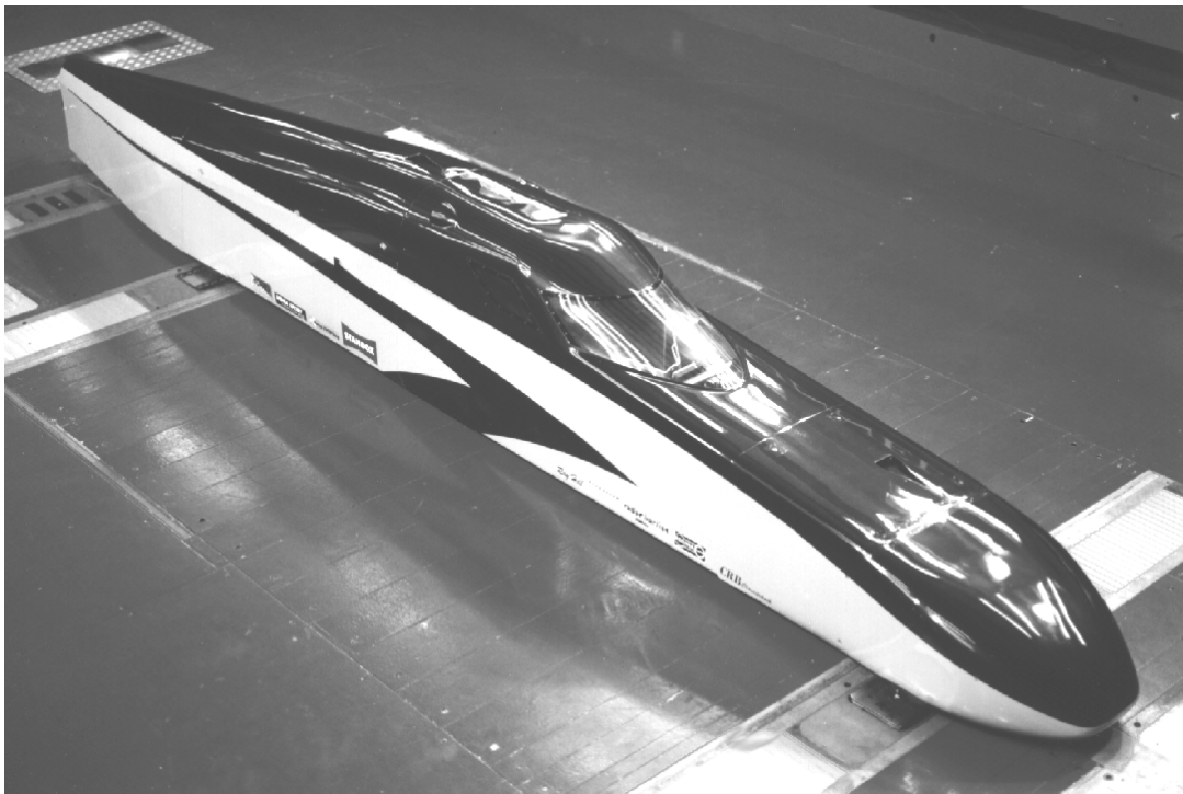
Figure 1. The Dreamliner III in the Volvo PVT wind tunnel.
